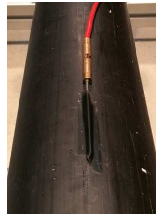
Figure 53: Glued PT-Element on the surface
